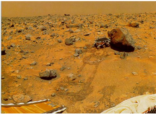
Mars Pathfinder (MESUR Pathfinder TM ) was an American spacecraft that landed a base station with a roving probe on Mars in 1997. It consisted of a lander , renamed the Carl Sagan Memorial Station, and a lightweight (10.6 kg/23 lb) wheeled robotic Mars rover named Sojourner
